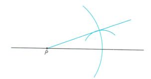
**3.** Construct a perpendicular to *CD* at *P*.
